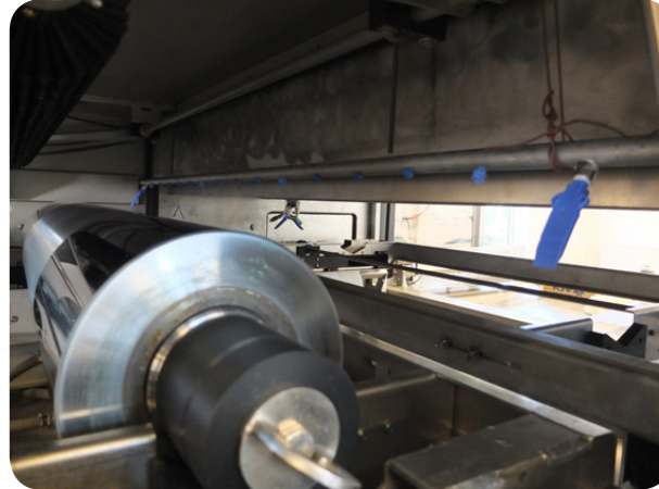
Spray arm and brushes inside the washing chamber
