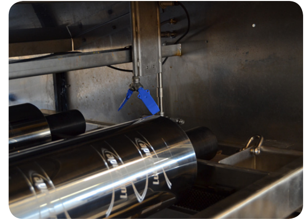
End brushes on carriage and high-pressure nozzles in rinse chamber
